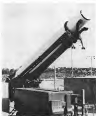
Thor intermediate range ballistic missile is moved half way to its launch position by a hoisting crane as preparation for firing from Vandenberg AFB launch site.
